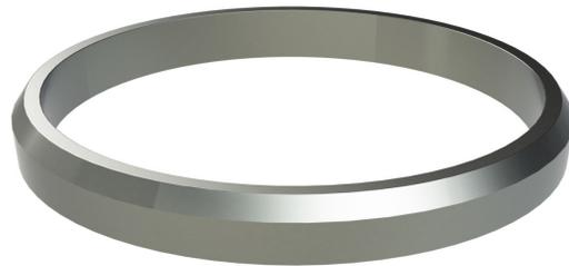
Due to the variation in drill pipe box sizes, Caproco offers corrosion rings in a variety of sizes and will custom manufacture rings to customer specifications. Post-exposure corrosion ring analysis is available, which includes accurate re-weighing, visual and pitting analysis and mpy wall-loss calculations provided in a concise report.
